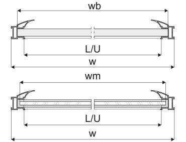
Dimensions helpful during installation of horizontal mid-rails in Simple 10 Frame systems
