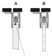
Expansion gap taken into account when calculating the height of chipboard
